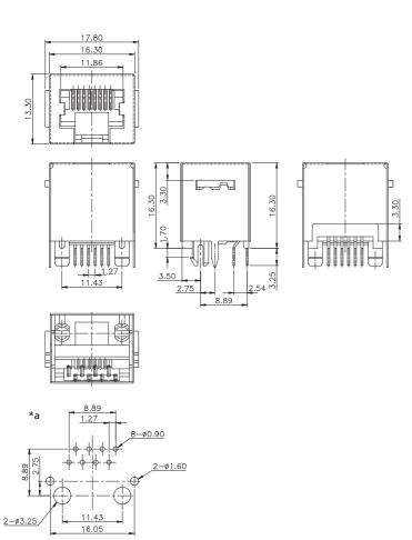
\*a printed circuit board layout, components side view
